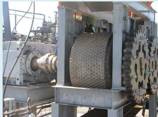
Roller on Briquetting machine
