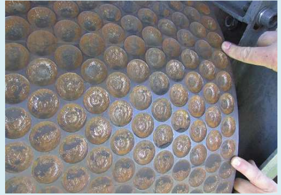
Bucket on roller of briquetting machine
